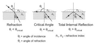
In the **MA871**, light from an LED passes through a prism in contact with the sample. An image sensor determines the critical angle at which the light is no longer refracted through the sample. The **MA871** automatically applies temperature compensation to the measurement and converts the refractive index of the sample to sucrose concentration in units of percent (by weight) Brix.
