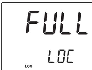
If the LOG/CLR/MR key is pressed while in measurement mode, a complete set of information is stored.
