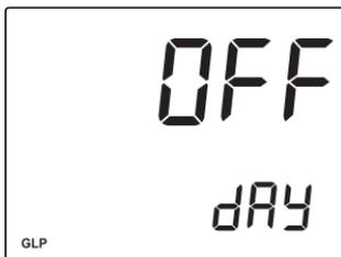
or the number of days before the calibration alarm will be displayed (e.g. 5 days), or from the time calibration expired (e.g. -3 days).
