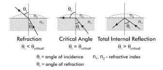
In the MA882, MA883, MA884 and MA885 refractometers, light from an LED passes through a prism in contact with the sample. An image sensor determines the critical angle at which the light is no longer refracted through the sample.
